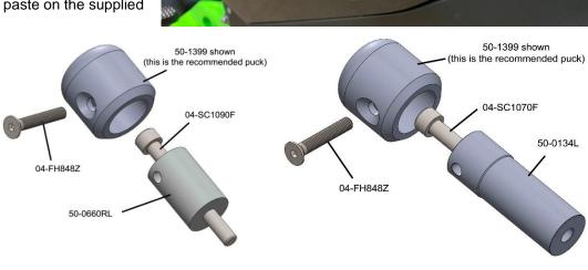
3) Attach the left slider base 50-0134L using the 10x70mm bolt.
