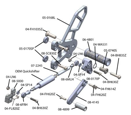
6) Remove the OEM shift knuckle and replace it with the ZX10 GP shift knuckle.
