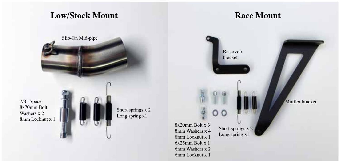
**Step 1:** Remove stock muffler and mid-pipe, as per owner's manual.
