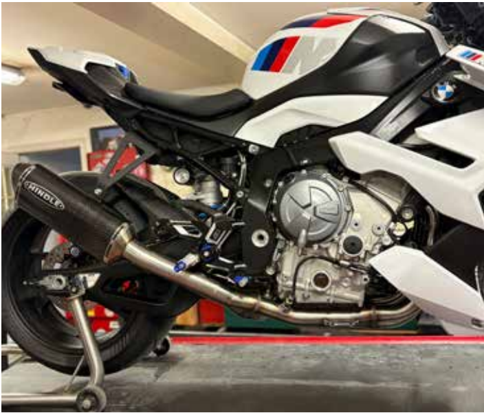
MUFFLER INSTALLED WITH RACE BRACKET
