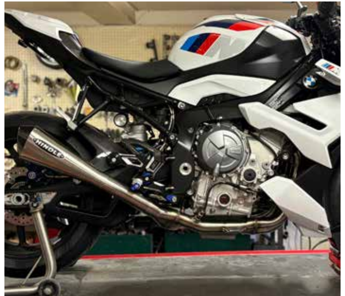
MEGAPHONE INSTALLED WITH FOOTPEG BRACKET
